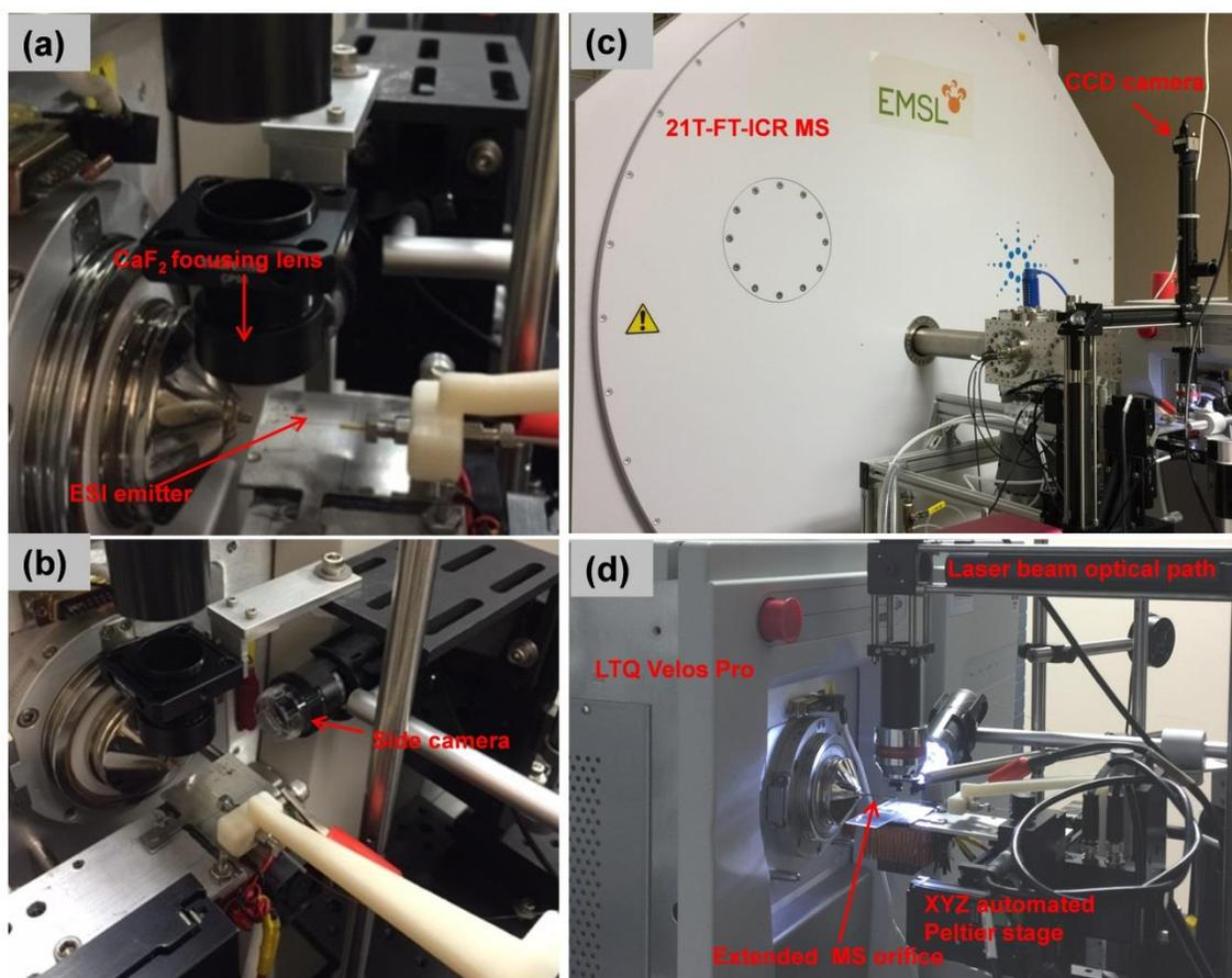
**Figure S3.** (a-b) Images of homebuilt LAESI source coupled to an LTQ Orbitrap Velos system used for source development. (c-d) Images of LAESI source coupled to a 21T-FTICR-MS housed at EMSL (see diagram in Figure 1).
